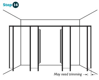
Repeat for the remaining Stiles and Fascias. Check the last Fascia before fixing as it may need trimming.
