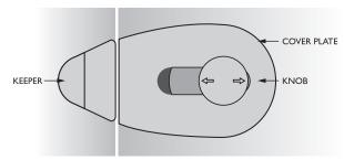
Then clip on the cover plate. Push on the knob and tighten the grub screws with the allen key supplied. A keeper will already be installed on the Stile.
