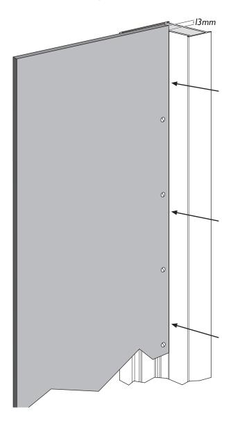
Push aluminium bead to click in place. (use additional polymer as required).
