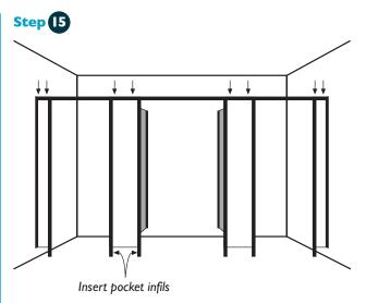
Fix Fascia panels in place, screw fix Headrail into the top of the full stiles.
