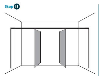
**Headrail** - Sit in place. This may require trimming as Headrails are supplied oversize. As Headrails are predrilled, make sure any trimming is done at the correct end - there will be a sticker to indicate which end.
