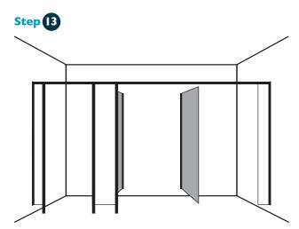
Place the next full stile into position and fix in place. Check the 'Resco shop drawings' to ensure that the full stile is orientated correctly.
