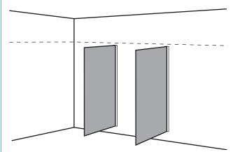
Place division panels into rear U-Channels with 4x2 blocks underneath to make them level (wedges will be required).
