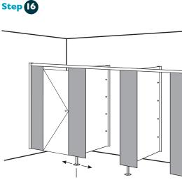
Adjust pedestals so that the gap is consistent.
