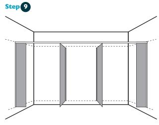
Place the Head rail on, ensuring flush with the walls.
