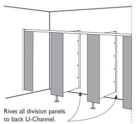
Use 3.5mm drill bit with (D) Stainless Steel Pop Rivets 30mm and 600mm from the top and the same from the bottom.
