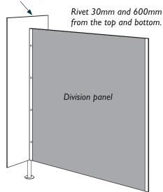
Finish riveting Fascias to division panels (rivet from the top down, 30mm and 600mm then up from the bottom 30mm and 600mm).
