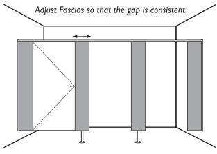
Close door, and adjust top as necessary to make the gap the same, then rivet through the top.
