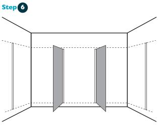
Fix side U-Channels (1795mm) flush with Datum and centered on Marks. The U-Channels are predrilled. Ensure screws go into wall frame.
