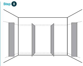
Place hinged Fascia into side U-Channels and align at the bottom.
