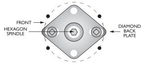
Fix the front part of the indicator bolt to the outside of the door using the diamond back plate on the inside of the door.
