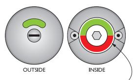
Insert the green and red plate into the inside of the front component of the indicator bolt.
