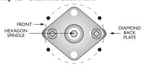
Fix the front part of the indicator bolt to the outside of the door using the diamond back plate on the inside of the door.
