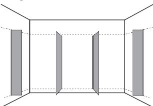
Place hinged Fascia into side U-Channels and align at the bottom. Ensure Plumb, and then fix on the inside of the cubicle with 4 Rivets, 30mm and 600mm down from the top, and the same up from the bottom.
