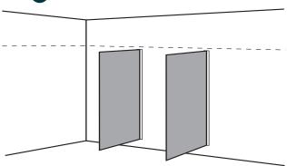
Place division panels into rear U-Channels with 4"x2" blocks underneath to make them level (wedges will be required). Ensure flush with the top of the U-Channel.
