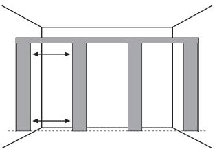
Starting with the Hinged Side Fascia, ensure that the door gap at the bottom is the same as the top gap.
