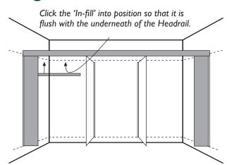
Starting at the hinge Fascia, insert first Door Infill into Headrail.
