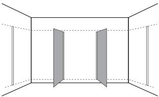
Fix side U-Channels (1795mm) flush with Datum and centred on marks. The U-Channels are predrilled. Ensure screws go into wall frame.
