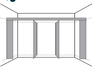
Trim the Headrail to ensure flush with the walls and position on to the top of the Side Fascias.
