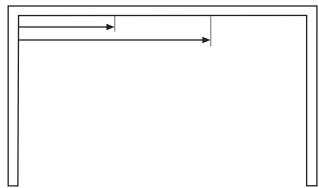
From the plans, mark the division centres on the back wall. Check location of toilets and ensure centred (these are sometimes fitted different to the plans).
