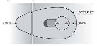
Then clip on the cover plate. Push on the knob and tighten the grub screws with the allen key supplied. Finally Fix the keeper on the fascia.
