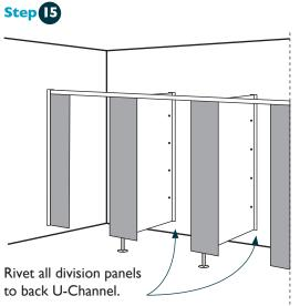
Use 3.5mm drill bit with (D) Stainless Steel Pop Rivets 30mm and 600mm from the top and the same from the bottom.
