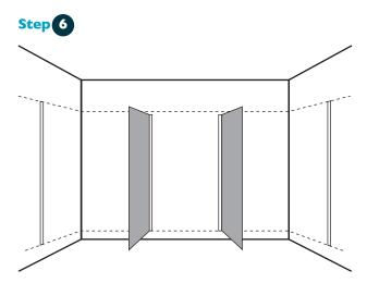
Fix side U-Channels (1795mm) flush with Datum and centered on Marks. The U-Channels are predrilled. Ensure screws go into wall frame.
