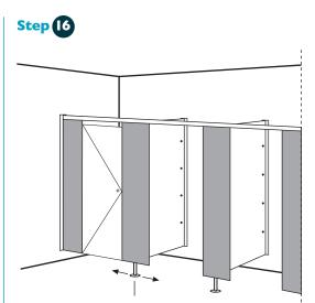
Adjust pedestals so that the gap is consistent.
