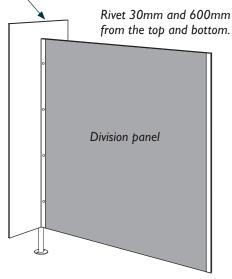
Finish riveting Fascias to division panels (rivet from the top down, 30mm and 600mm then up from the bottom 30mm and 600mm).
