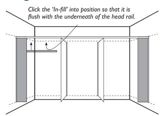
Starting at the hinge Fascia, insert first Door Infill into Head rail.
