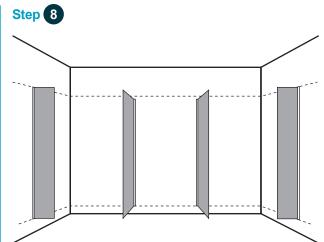
Place hinged Fascia into side U-Channels and align at the bottom.
