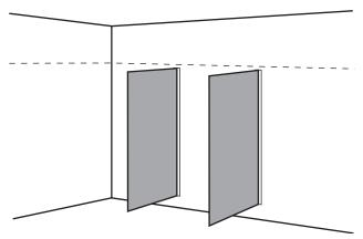
Place division panels into rear U-Channels with 4x2 blocks underneath to make them level (wedges will be required).
