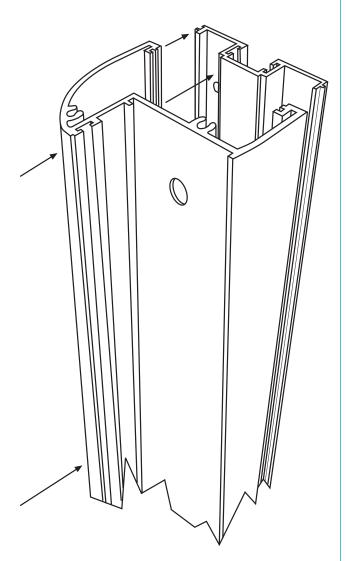
Clip 1/2 Stile to bracket and fix through holes with 3 x 2" screws.
