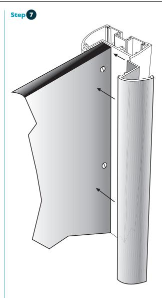
Quickly, before the Polymer dries, clip the corner bead in place.
