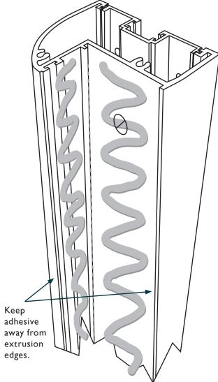
Place MS Polymer adhesive along the ½ Stile back and the side as shown.
