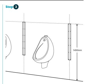
Attach wall bracket by screw fixing in place using 11/4" screws centered on the marks with 6 screws through the outside holes.
